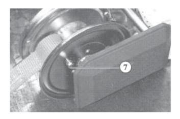
Insert and tighten the screw complete with washer (7) through the outside of the drum into the threaded hole in the anchor bar
