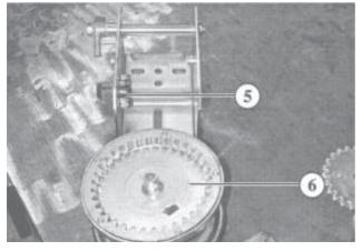
• To remove the intermediate pinion (5), remove the drum (6)
