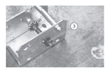
• Fit the bush (3) onto the drive shaft and press into the housing
