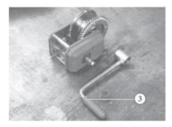
• Loosen and take off the crank handle (3) by turning to the left several times
